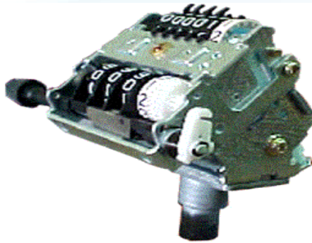
Fig.2. Angular drive Speedo movements
