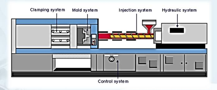
The injection machine is a machine that melt plasticize the molding material inside the heating cylinder and inject this into the mold tool / Cavity to create the molded product by solidifying inside it.
